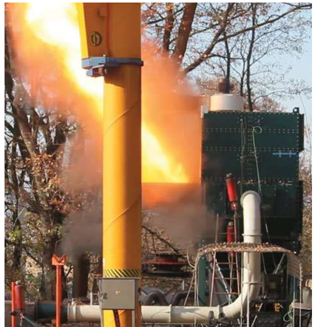
An engineered test is performed at an official testing facility to confirm that the dust collector can withstand an explosive event.
